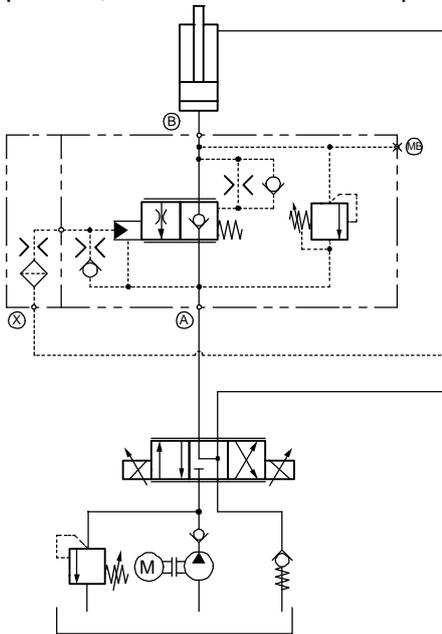
Circuit example for SVZ (B → L), not influenced by return-line pressure, for directional valves with closed-centre spool
