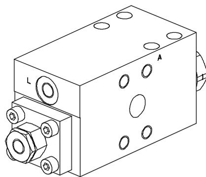
The main port is defined as seen from the perspective of the cover. As standard, the main port A is located on the right side. A variant with main port A1 is available as an option.
